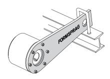
The Model FRB clutches must be secured to the shaft by customer supplied snap ring, set collar, spacer, etc. All fasteners are recommended to be grade 8.
